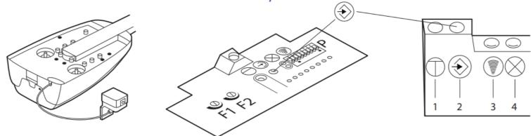
Locate the button on the motor of CRAWFORD. Press briefly the button the release it. The LED lightens up.
