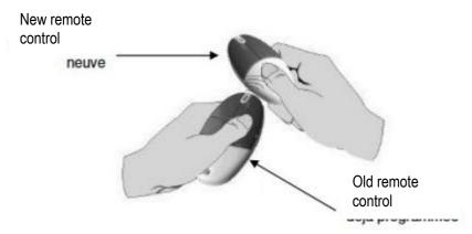
Press the button on your old remote control. The new remote control flashes 3 times
