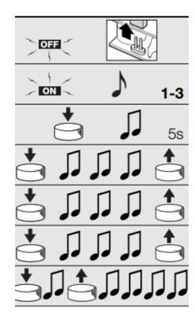
When the memory contains no transmitters the first one can be memorized in mode II as follows:
