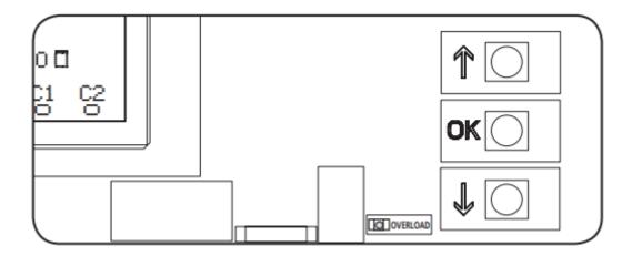
By pressing OK button you can access the programming and configuration menus of each individual parameters
