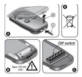
First check that the transmitter is operating by pressing one of its buttons and check that the Led flashes at the same time (= transmission performed).
