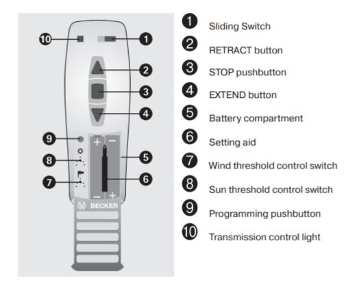
Before programming the radio, check if the threshold actuator is set on factory setting. When Programming the transmitter, make sure you are not close to the operating area of the sun protection system.
