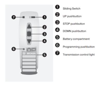
**NOTE**: Before entering this MC441 transmitter, make sure that a master transmitter has been already programmed into the receiver and the motor has learned the upper and lower stops.
